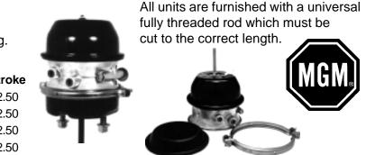
MGM Model TR-TS Series -(30/30 combo 2.5" stroke) "Full Epoxy Coated External Tube Breather System." The power spring chamber is "sealed" against any contaminated and corrosive outside air because 100% of the air drawn in originates from the inside protected area of the service brake chamber. The result is an MGM spring brake that is CORROSION-FREE... proven in over 25 years of use on heavy vehicles of European origin equipped with MGM-Europa spring brakes. Same for the MGM Model LTR-T Series.
